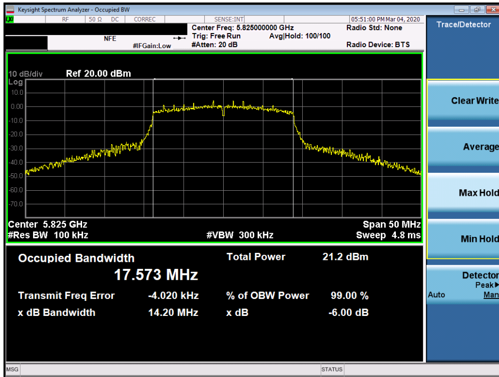
Plot 7-36. 6dB Bandwidth Plot (20MHz BW 802.11n (UNII Band 3) – Ch. 165)
