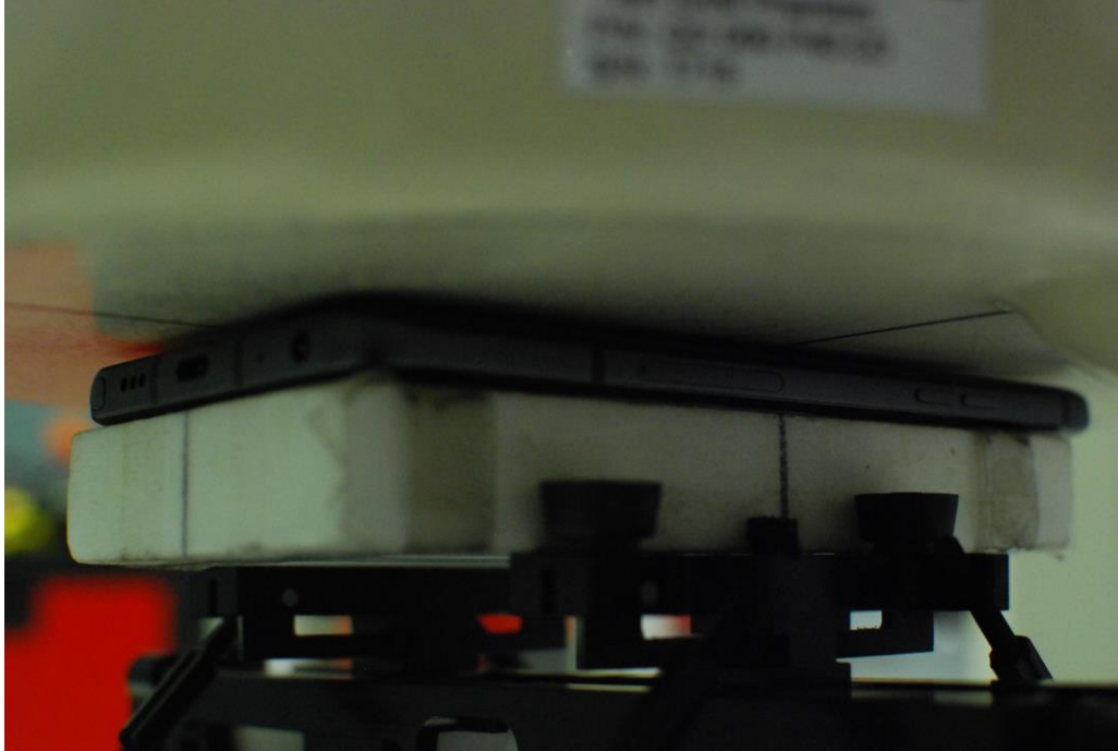
SAR Test Setup Photo 17 –Back Side at 1 mm
