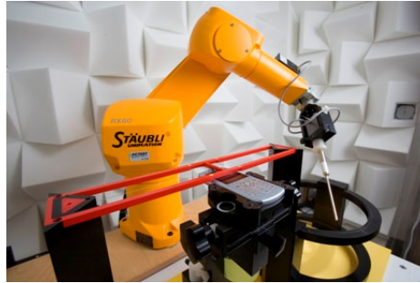
Figure 4-3 SPEAG Robotic System
