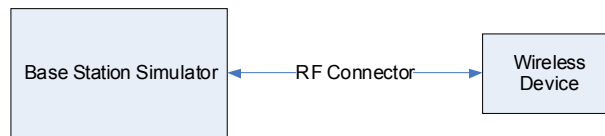
Figure 9-1 Power Measurement Setup
