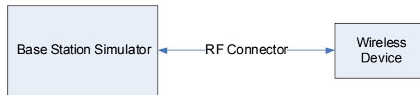
Figure 9-2 Power Measurement Setup
