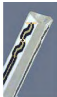
Figure 3.3 Probe Thick-Film Technique
