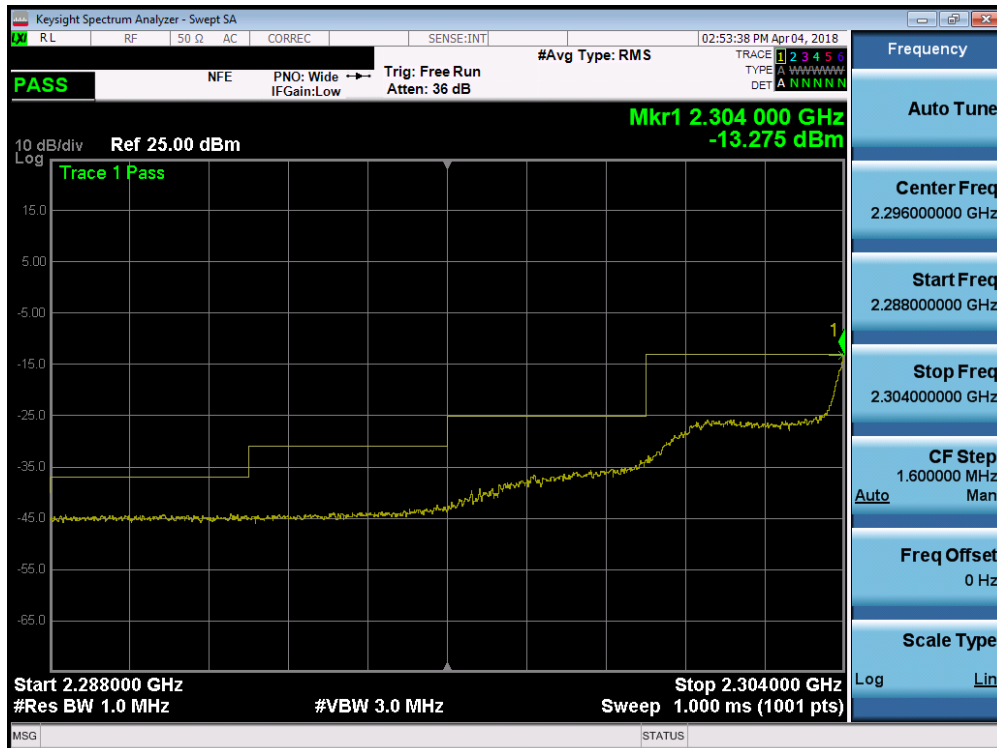
Plot 7-149. Lower Extended Band Edge Plot (Band 30 - 5.0MHz QPSK - Full RB Configuration)
