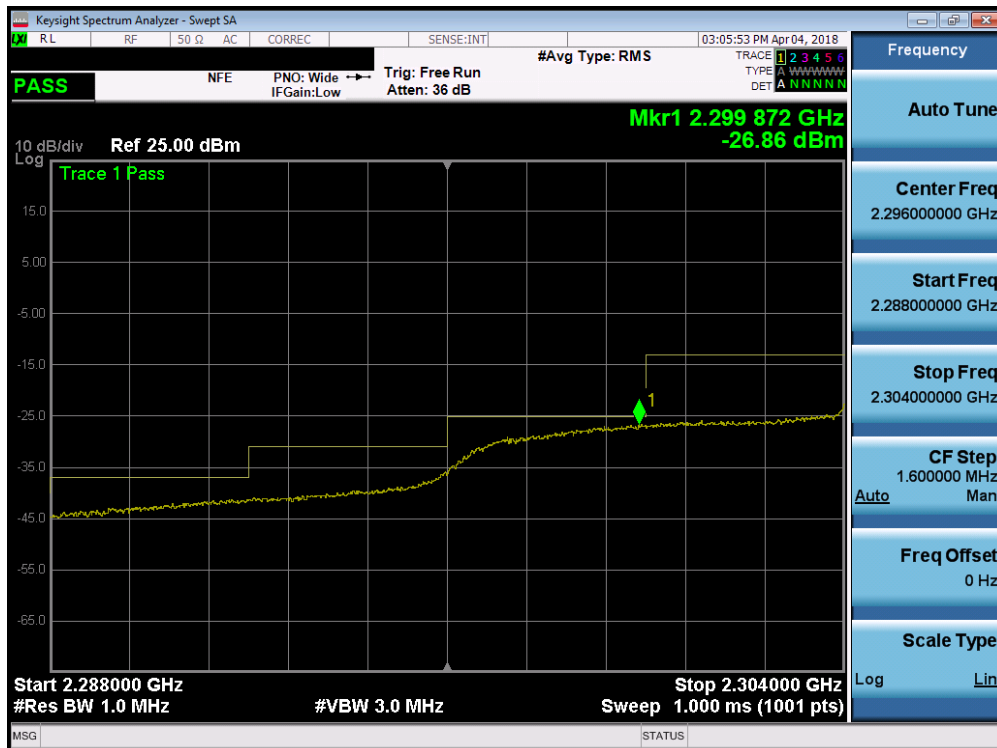
Plot 7-153. Lower Extended Band Edge Plot (Band 30 - 10.0MHz QPSK - Full RB Configuration)
