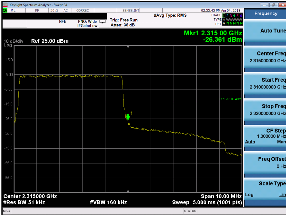
Plot 7-150. Upper Band Edge Plot (Band 30 - 5.0MHz QPSK - Full RB Configuration)
