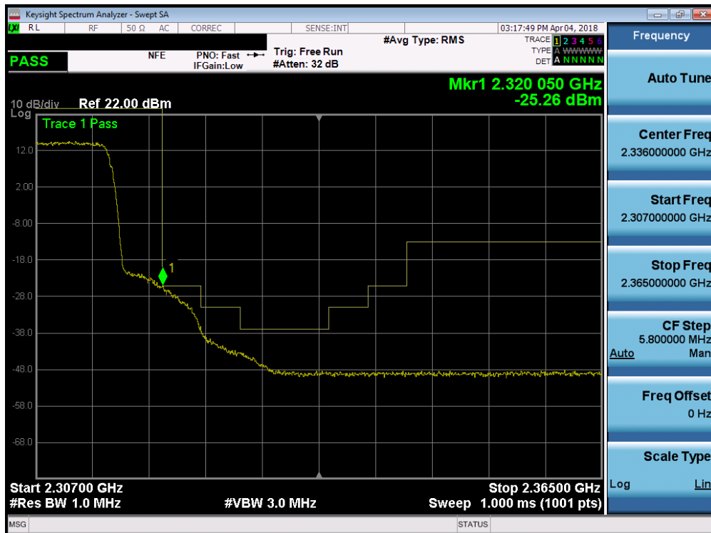
Plot 7-155. Upper Extended Band Edge Plot (Band 30 - 10.0MHz QPSK - Full RB Configuration)
