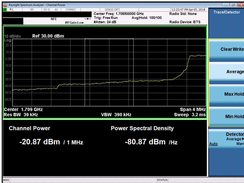
Plot 7-105. Lower Extended Band Edge Plot (Band 4 - 3.0MHz QPSK - Full RB Configuration)
