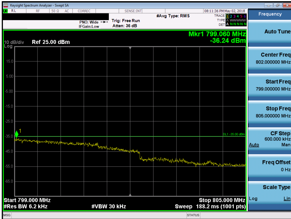
Plot 7-11. Upper Emission Mask Band Edge Plot (Band 14 - 5.0MHz QPSK - Full RB Configuration)
