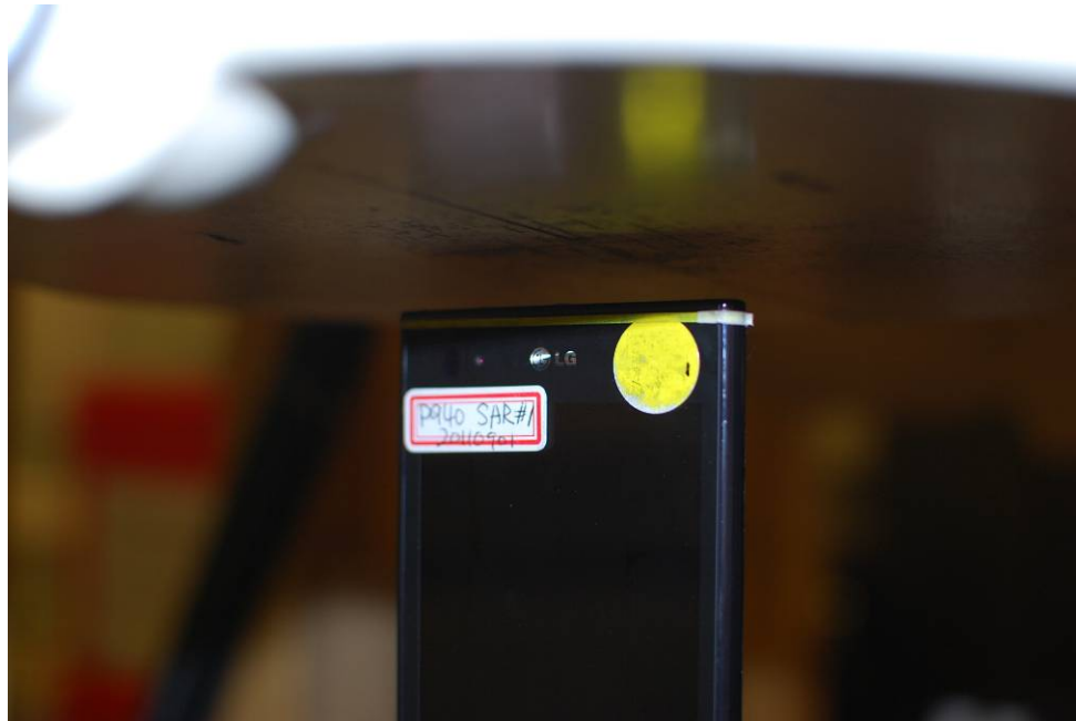
SAR Test Setup Photo 7 – Top at 1.0 cm
