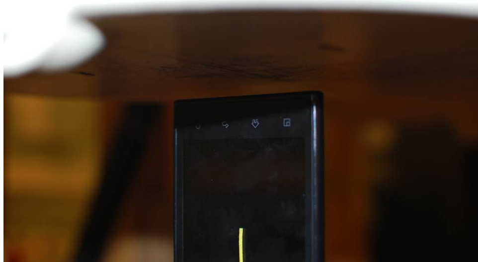
SAR Test Setup Photo 8 – Bottom at 1.0 cm
