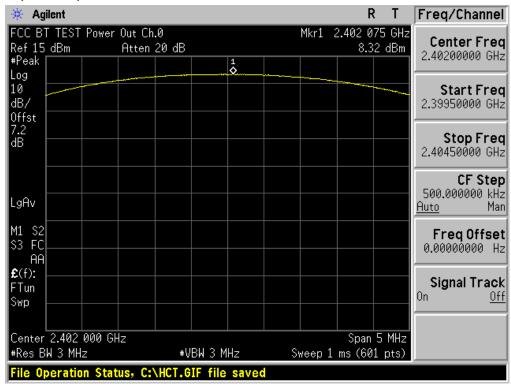
Test Plots (π/4DQPSK) Peak Power (Mid-CH)
