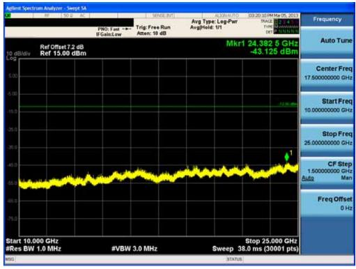
Test Plots ( $\pi$ /4DQPSK) - 10 GHz - 25 GHz (RBW:1 MHz, VBW: 1 MHz) Spurious Emission (Mid-CH)
