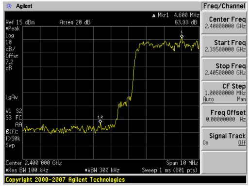
Test Plots with hopping ( $\pi$ /4DQPSK) Band Edges (High-CH)
