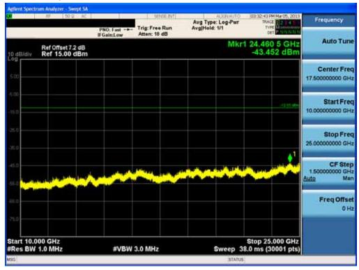
Test Plots (8DPSK) - 10 GHz - 25 GHz (RBW:1 MHz, VBW: 1 MHz) Spurious Emission (Low-CH)
