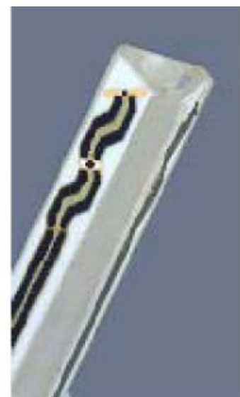
Figure 3.3 Probe Thick-Film Technique
