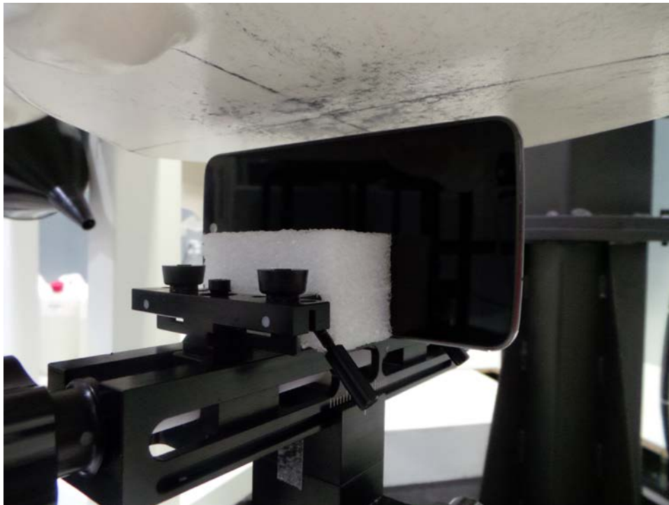
SAR Test Setup Photo 10: Left Edge at 1.0 cm
