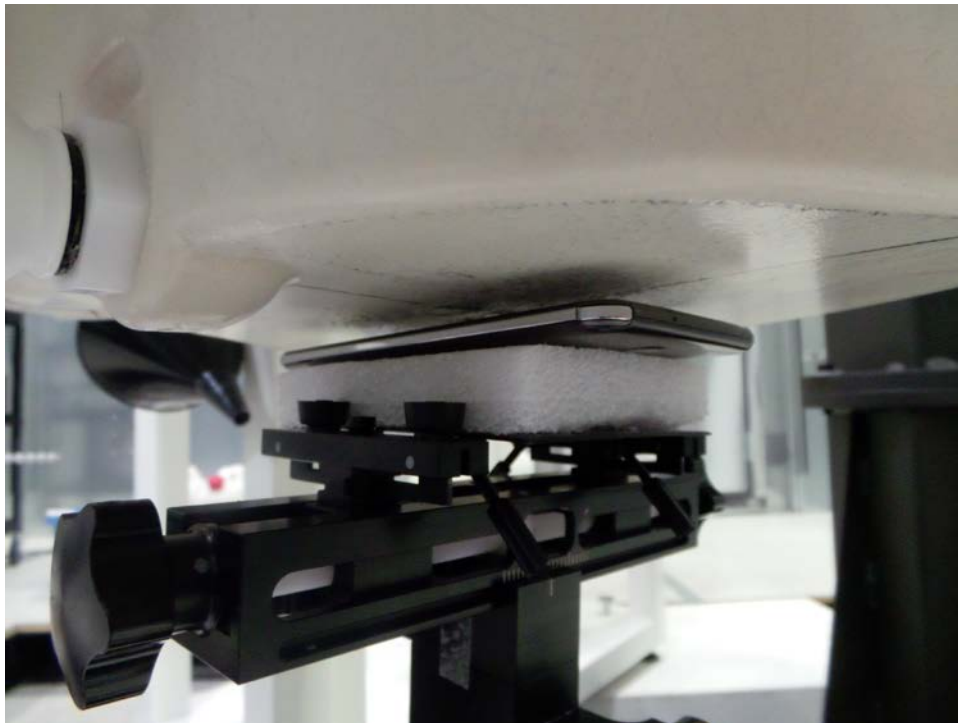
SAR Test Setup Photo 6: Front Side at 1.0 cm
