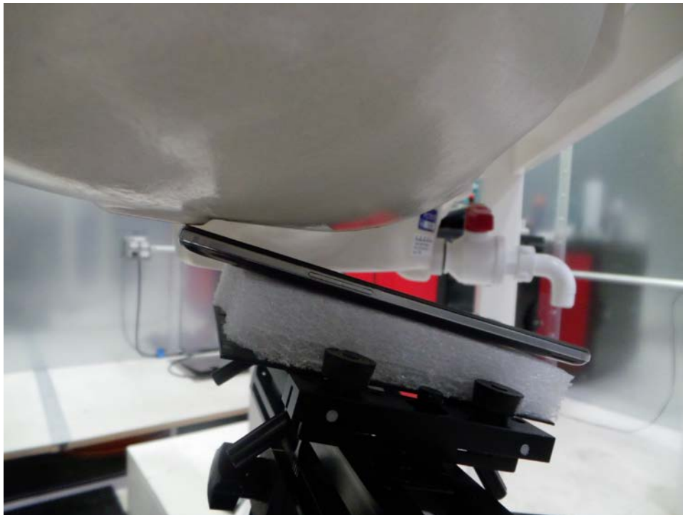
SAR Test Setup Photo 2: Right Tilt
