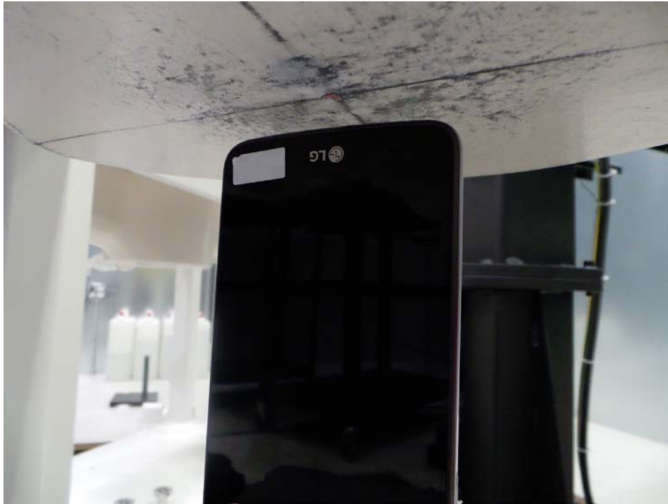
SAR Test Setup Photo 8: Bottom Edge at 1.0 cm
