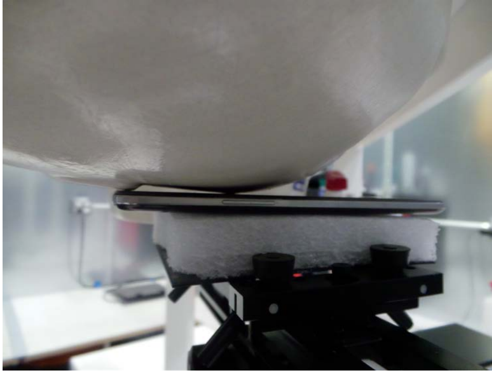
SAR Test Setup Photo 1: Right Cheek
