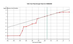
This model was verified to be within the linear region for ABM1 measurements at -18 dBm0 for CDMA. This measurement was taken in the axial configuration above the maximum location.
