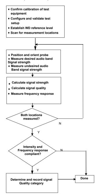
Figure 4-16 C63.19 T-Coil Signal Test Process
