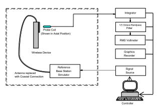
Figure 4-14 Audio Magnetic Field Test Setup
