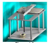
Figure 4-3 RF Near-Field Scanner
