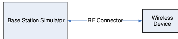
Figure 9-3 Power Measurement Setup
