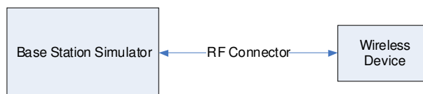
Figure 9-2 Power Measurement Setup
