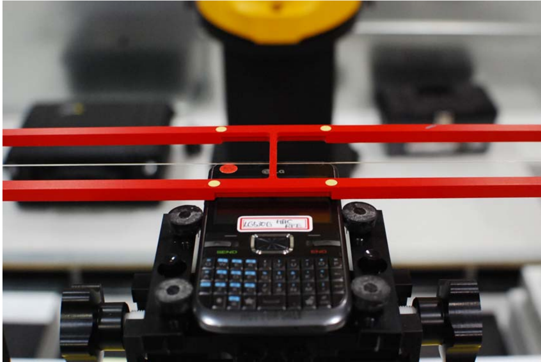
Figure 17-1 Ear Reference Point HAC Phantom Alignment
