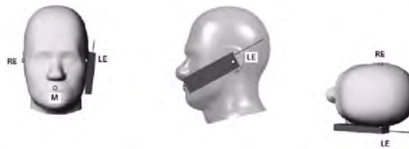
Figure 6.1 Front, Side and Top View of Cheek/Touch Position
