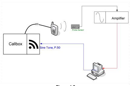
Figure 4-2 T-Coil Test Setup
