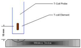
Figure 4-11 Measurement Distance
