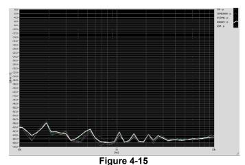
High power RF Emissions Effect with HAC Dipole on the T-coil Probe System 10mm between dipole maximum and magnetic probe
