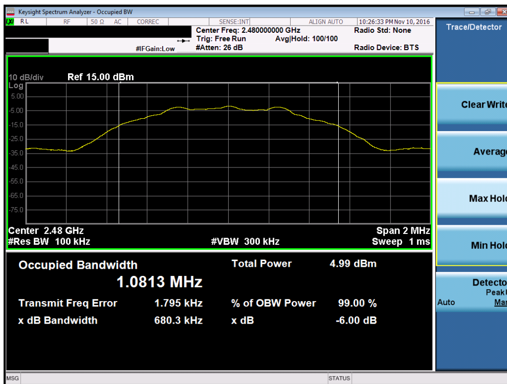
Plot 7-3. 6dB Bandwidth Plot (Bluetooth (LE) – Ch. 39)
