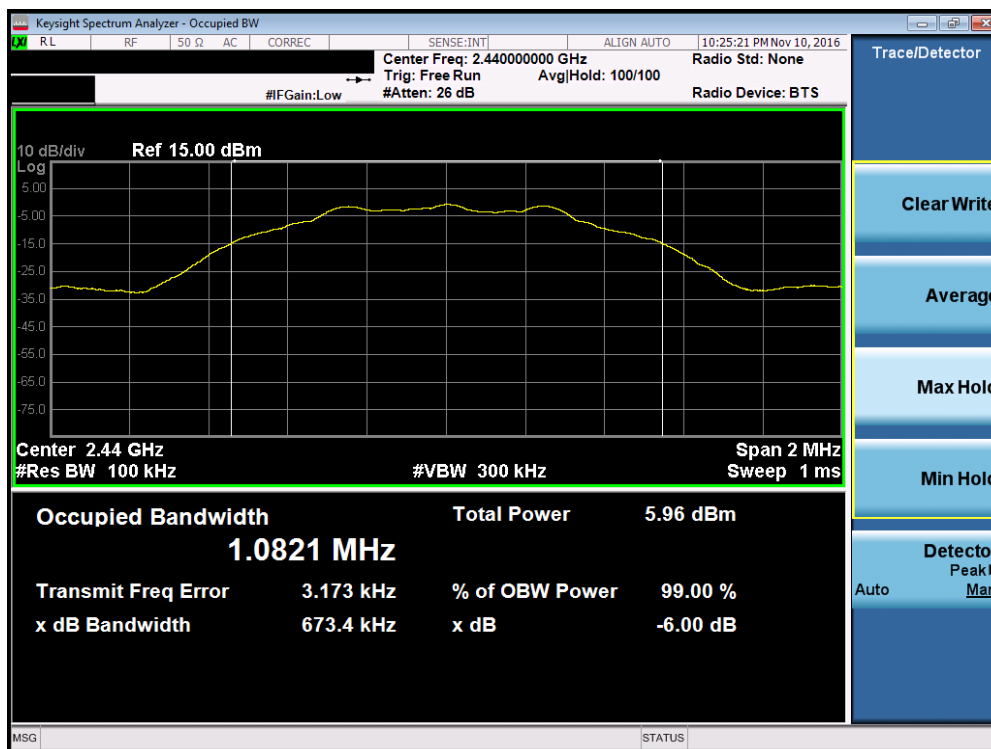
Plot 7-2. 6dB Bandwidth Plot (Bluetooth (LE) – Ch. 19)
