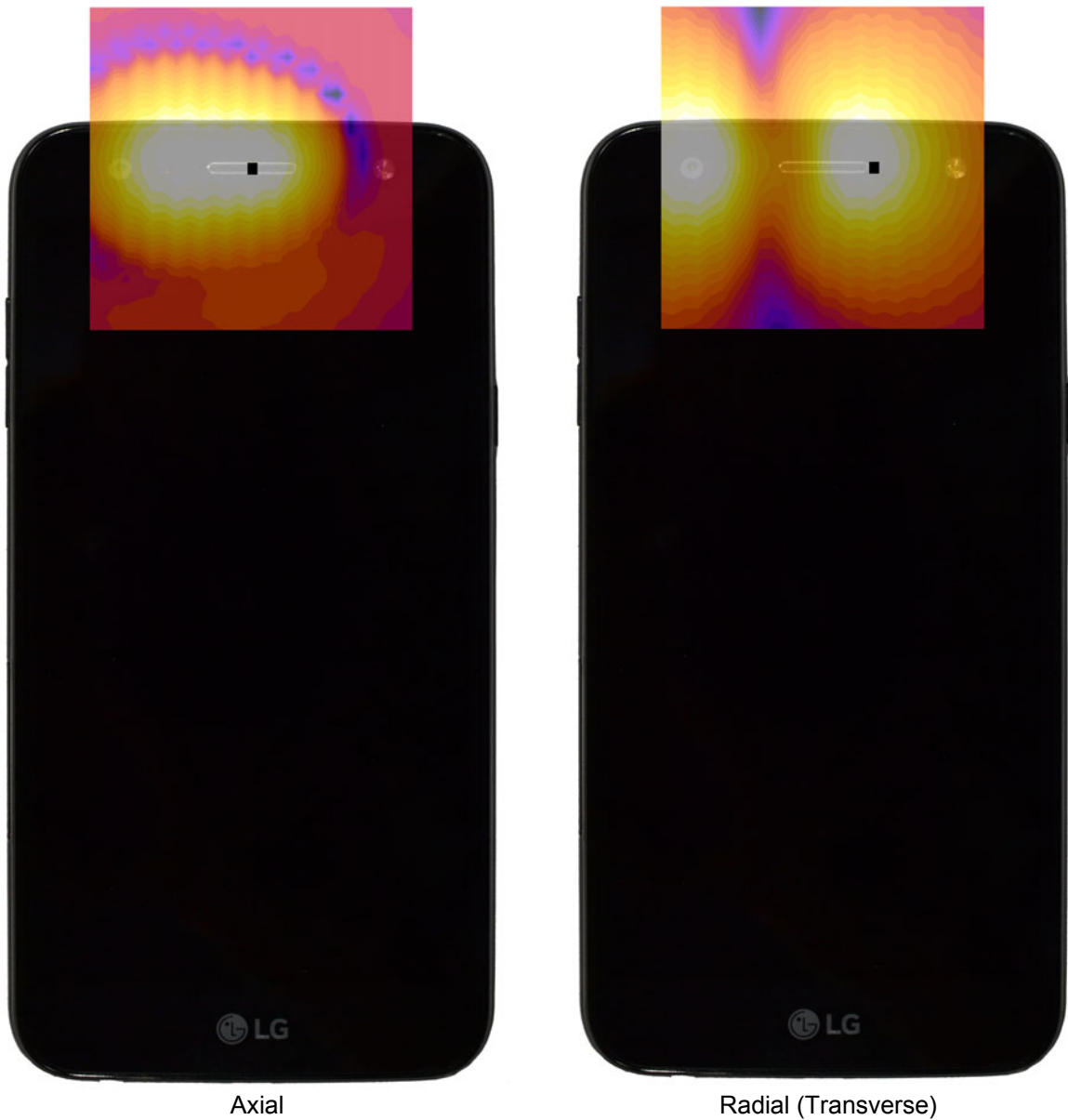
Figure 13-3 T-Coil Scan Overlay Magnetic Field Distributions
