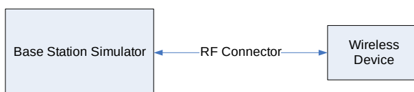
Figure 9-2 Power Measurement Setup
