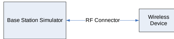
Figure 9-4 Power Measurement Setup
