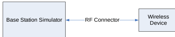
Figure 9-3 Power Measurement Setup
