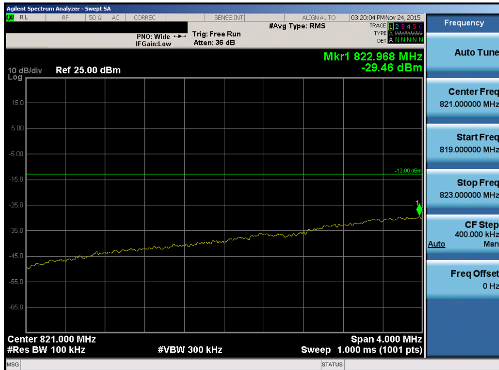
Plot 7-96. Lower Extended Band Edge Plot (Band 5 – 3.0MHz QPSK – RB Size 15)
