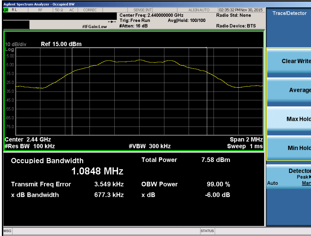
Plot 7-2. 6dB Bandwidth Plot (Bluetooth (LE) – Ch. 19)
