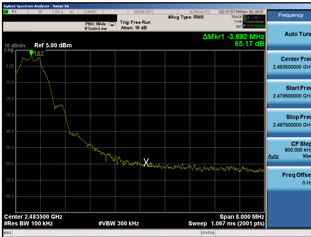
Plot 7-11. Band Edge Plot (Bluetooth (LE) – Ch. 39)
