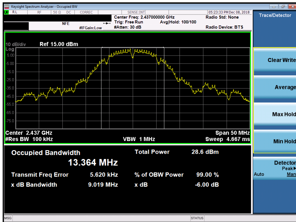
Plot 7-2. 6dB Bandwidth Plot (802.11b – Ch. 6)
