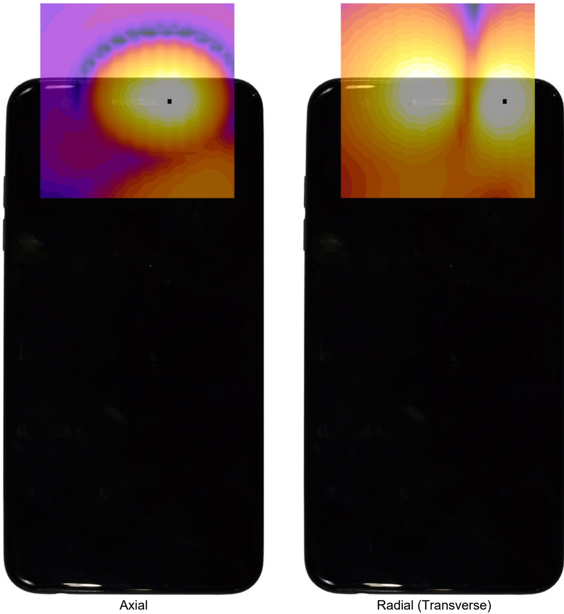
Figure 16-3 T-Coil Scan Overlay Magnetic Field Distributions
