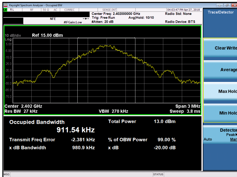
Plot 7-1. 20dB Bandwidth Plot (Bluetooth, 1Mbps – Ch. 0)
