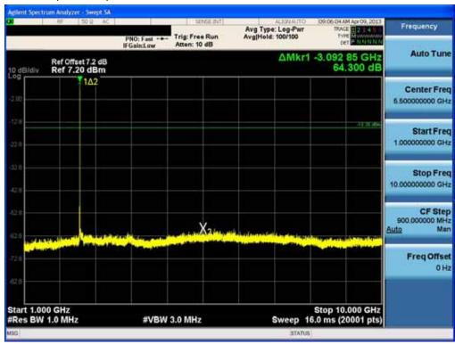
Test Plots ( $\pi$ /4DQPSK) - 1 GHz - 10 GHz (RBW:1 MHz, VBW: 1 MHz) Spurious Emission (Mid-CH)
