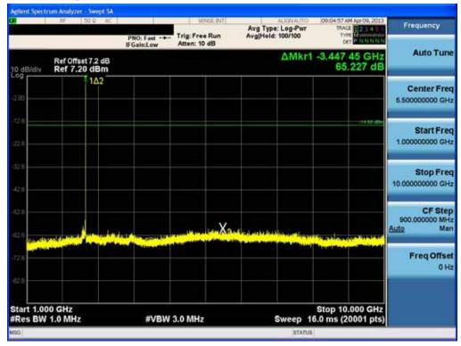
Test Plots (8DPSK) - 1 GHz - 10 GHz (RBW:1 MHz, VBW: 1 MHz) Spurious Emission (Low-CH)
