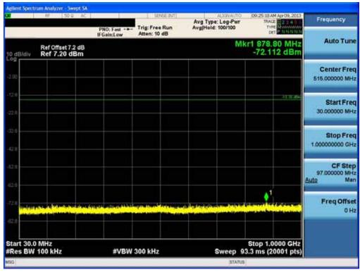
Test Plots ( $\pi$ /4DQPSK) - 30 MHz - 1 GHz (RBW:100 kHz, VBW: 300 kHz) Spurious Emission (Mid-CH)
