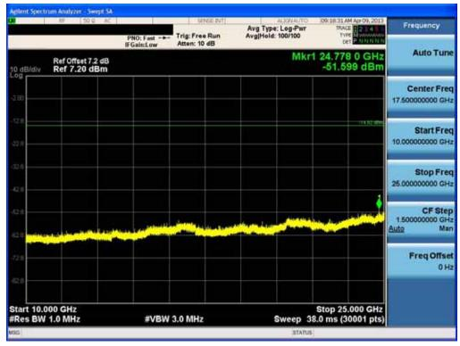
Test Plots (GFSK) - 10 GHz - 25 GHz (RBW:1 MHz, VBW: 1 MHz) Spurious Emission (Mid-CH)
