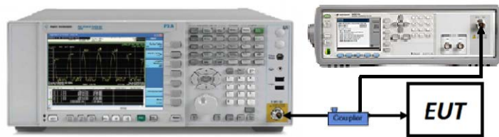
Figure 7-6. Test Instrument & Measurement Setup
