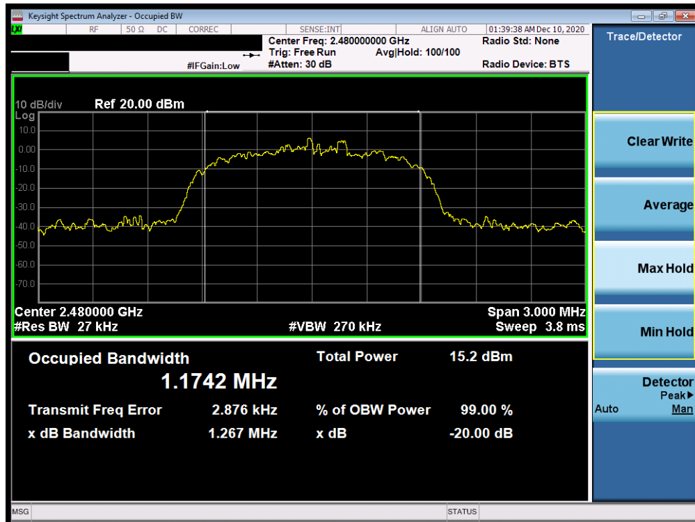
Plot 7-9. 20dB Bandwidth Plot (Bluetooth, 3Mbps – Ch. 78)
