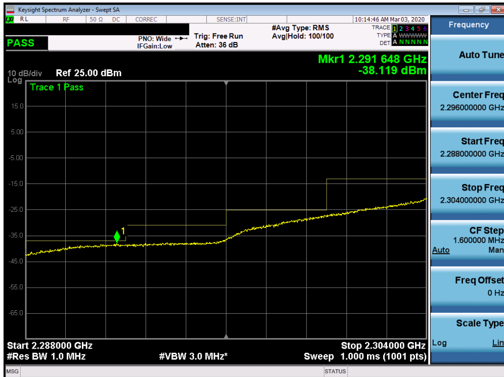
Plot 7-162. Lower Extended Band Edge Plot (Band 30 - 10.0MHz QPSK - Full RB Configuration)
