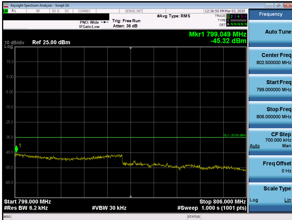
Plot 7-11. Upper Extended Band Edge Plot (Band 14 - 5MHz QPSK – Full RB Configuration)
