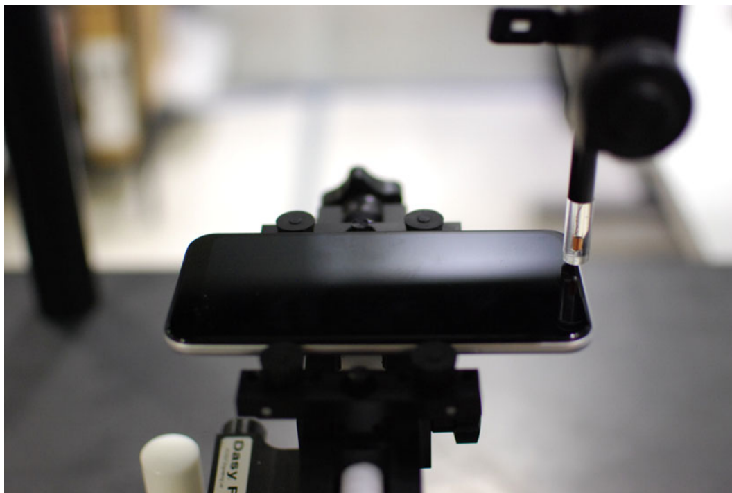
Figure 16-1 Test Setup for Wireless Device
