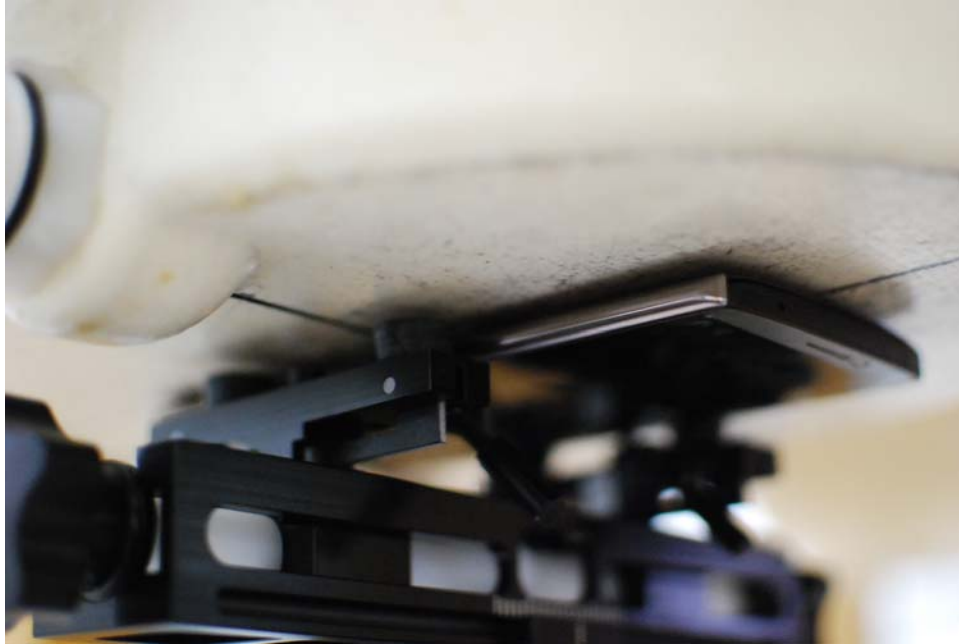
SAR Test Setup Photo 9: Back Side, Standard Cover at 0 mm
