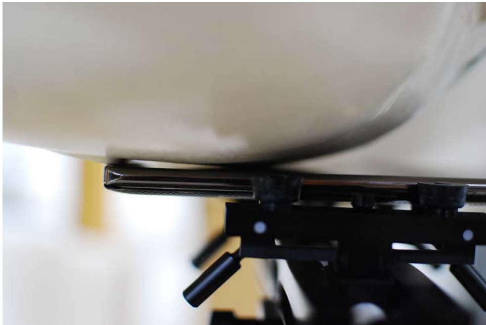
SAR Test Setup Photo 2: Right Cheek, Wireless Charging Cover
