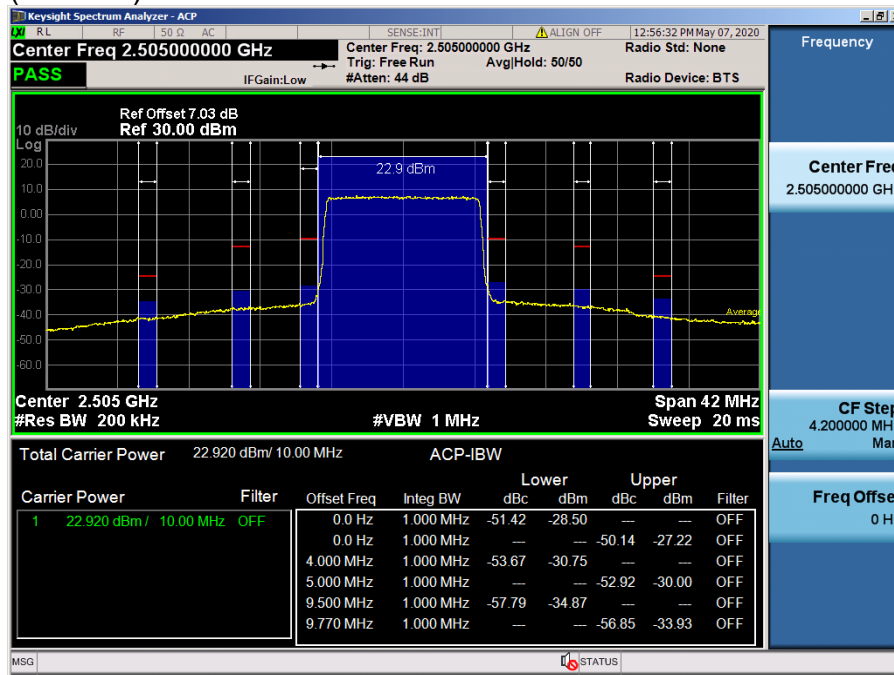
LTE Band 7 / 10 MHz / 16QAM - RB Size/Offset (50/0)
