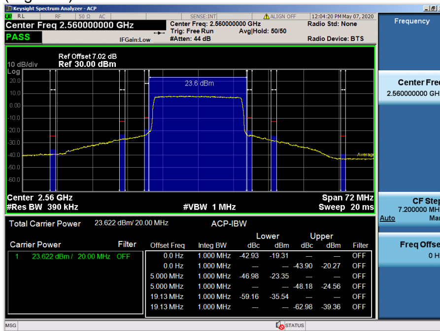
LTE Band 7 / 20 MHz / QPSK - RB Size/Offset (100/0)
