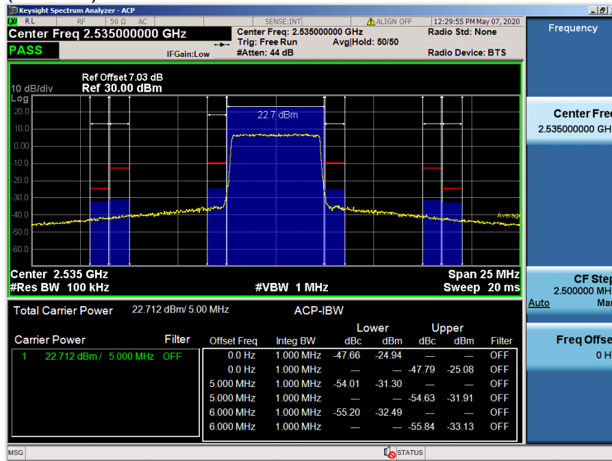
LTE Band 7 / 5 MHz / 16QAM - RB Size/Offset (25/0)
