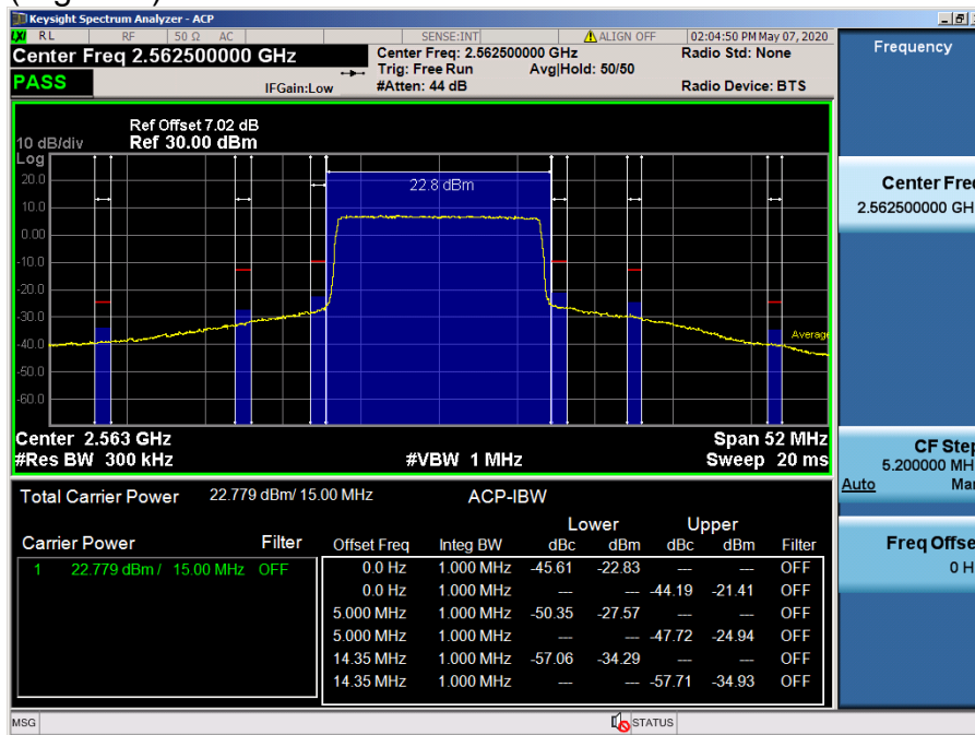
LTE Band 7 / 15 MHz / 16QAM - RB Size/Offset (75/0)
