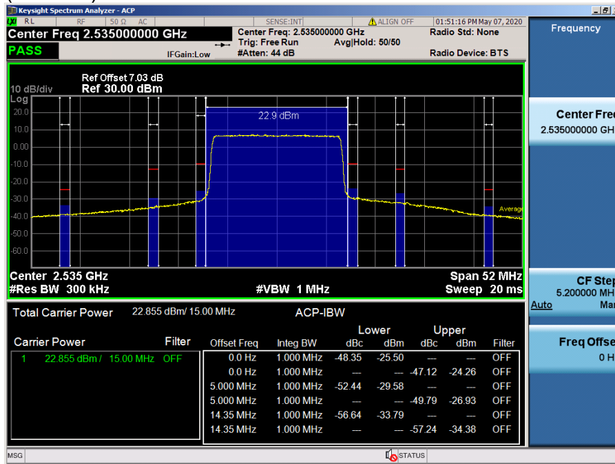
LTE Band 7 / 15 MHz / 16QAM - RB Size/Offset (75/0)
