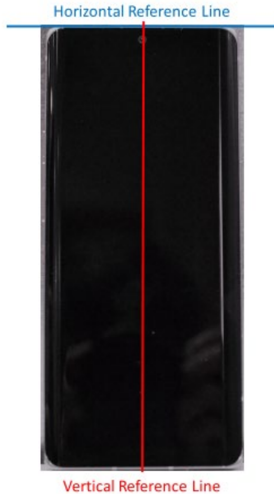
SAR Test Setup Photo 20: Horizontal and Vertical Reference Lines
