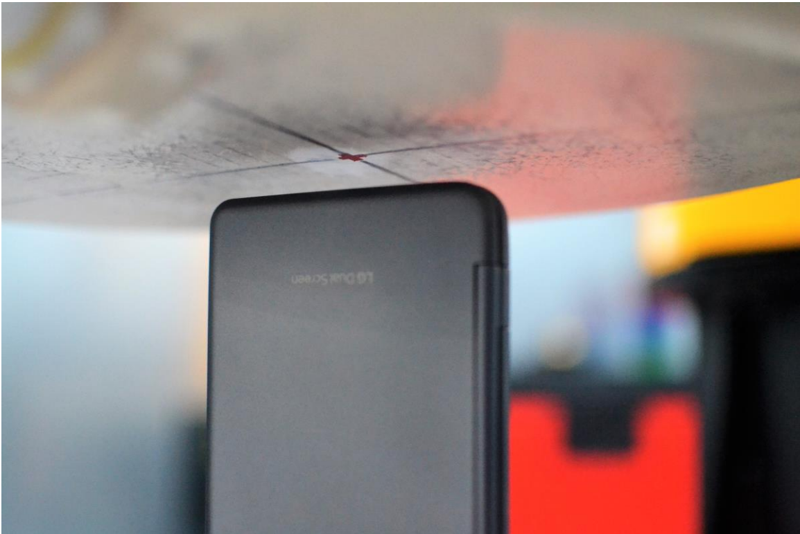
SAR Test Setup Photo 28 – Bottom Edge with Dual Display Accessory Position #1 at 10 mm
