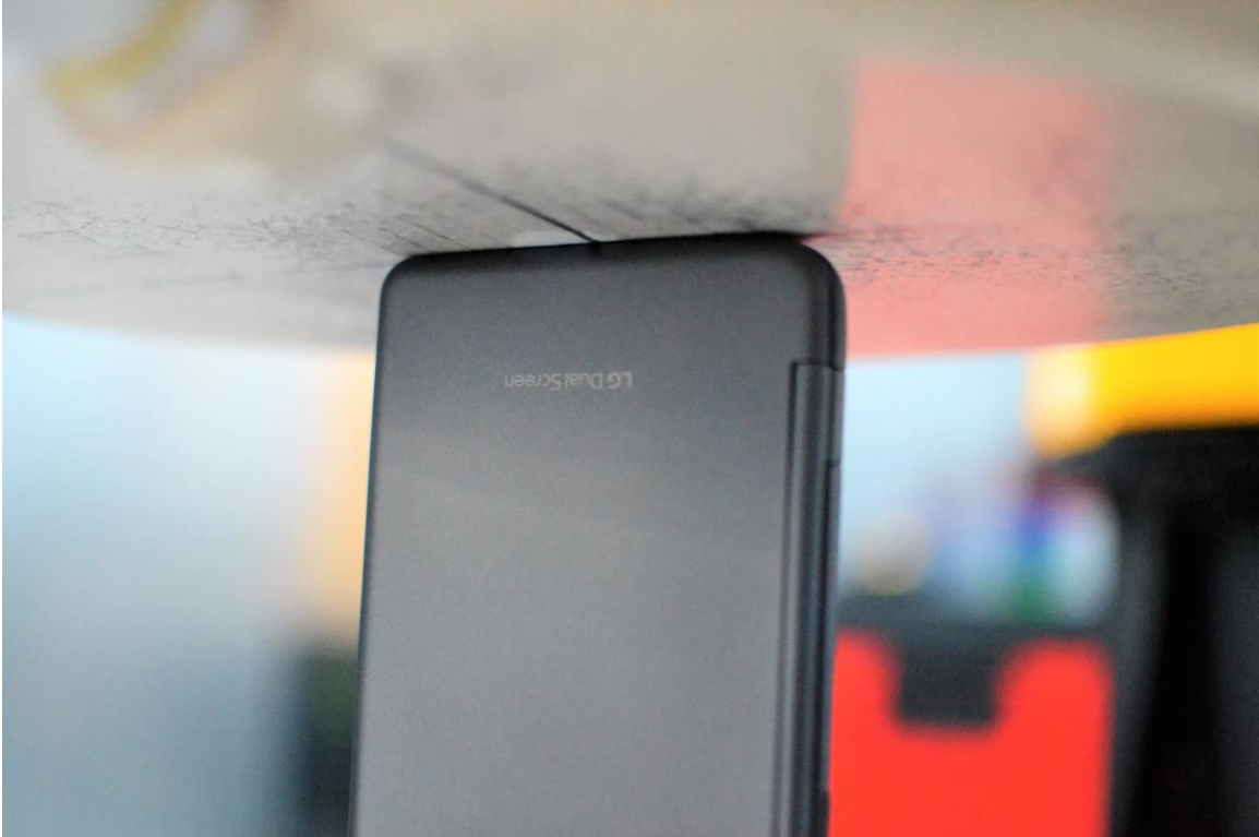
SAR Test Setup Photo 29 – Bottom Edge with Dual Display Accessory Position #1 at 0 mm
