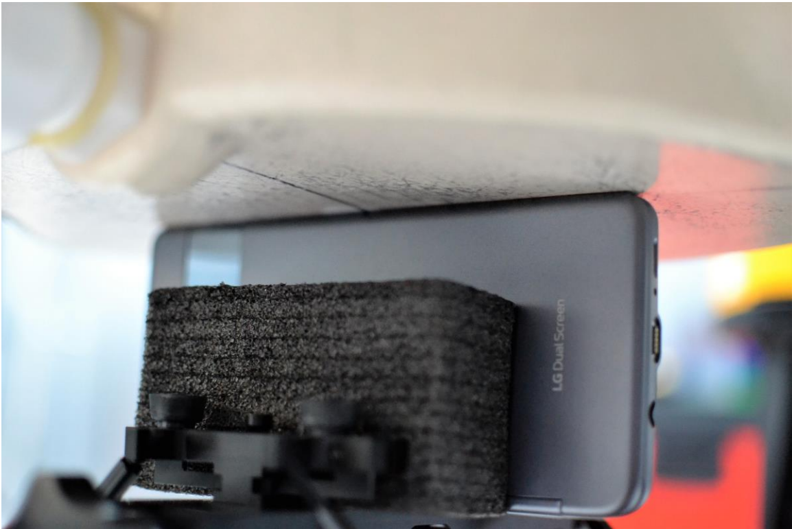
SAR Test Setup Photo 34 – Right Edge with Dual Display Accessory Position #1 at 0 mm
