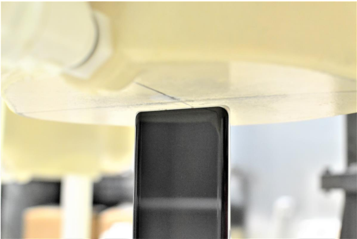
SAR Test Setup Photo 26 – Bottom Edge at 3 mm
