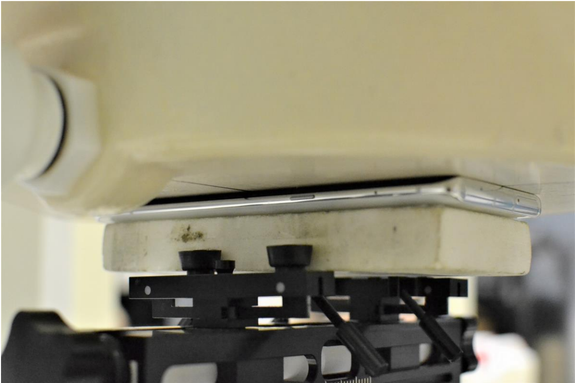
SAR Test Setup Photo 18 – Front Side at 0 mm
