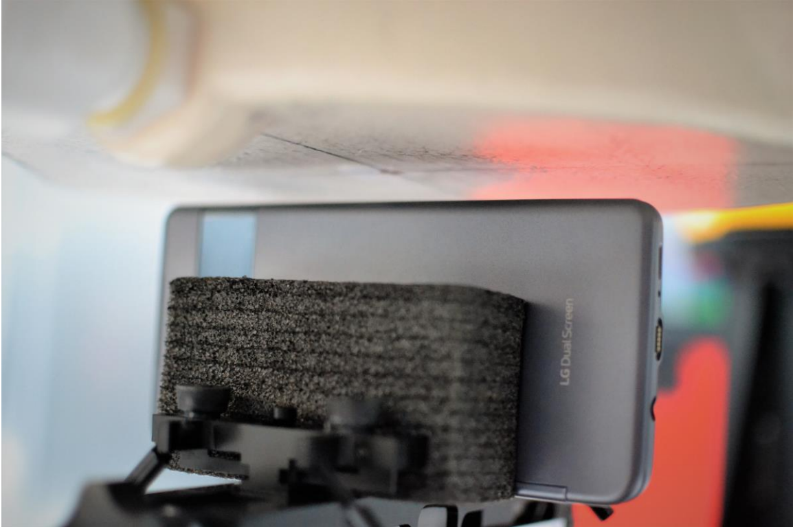
SAR Test Setup Photo 33 – Right Edge with Dual Display Accessory Position #1 at 10 mm
