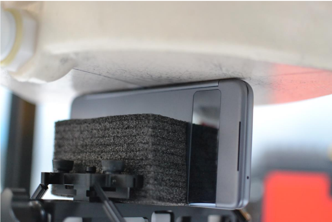
SAR Test Setup Photo 38 – Left Edge with Dual Display Accessory Position #1 at 0 mm
