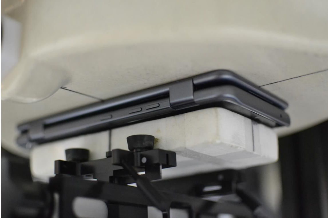
SAR Test Setup Photo 15 – Back Side with Dual Display Accessory Position #3 at 0 mm
