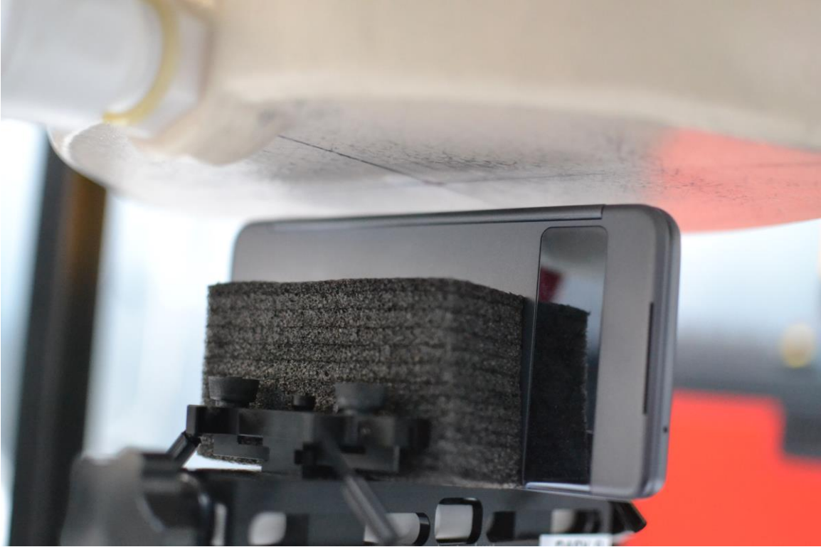
SAR Test Setup Photo 37 – Left Edge with Dual Display Accessory Position #1 at 10 mm
