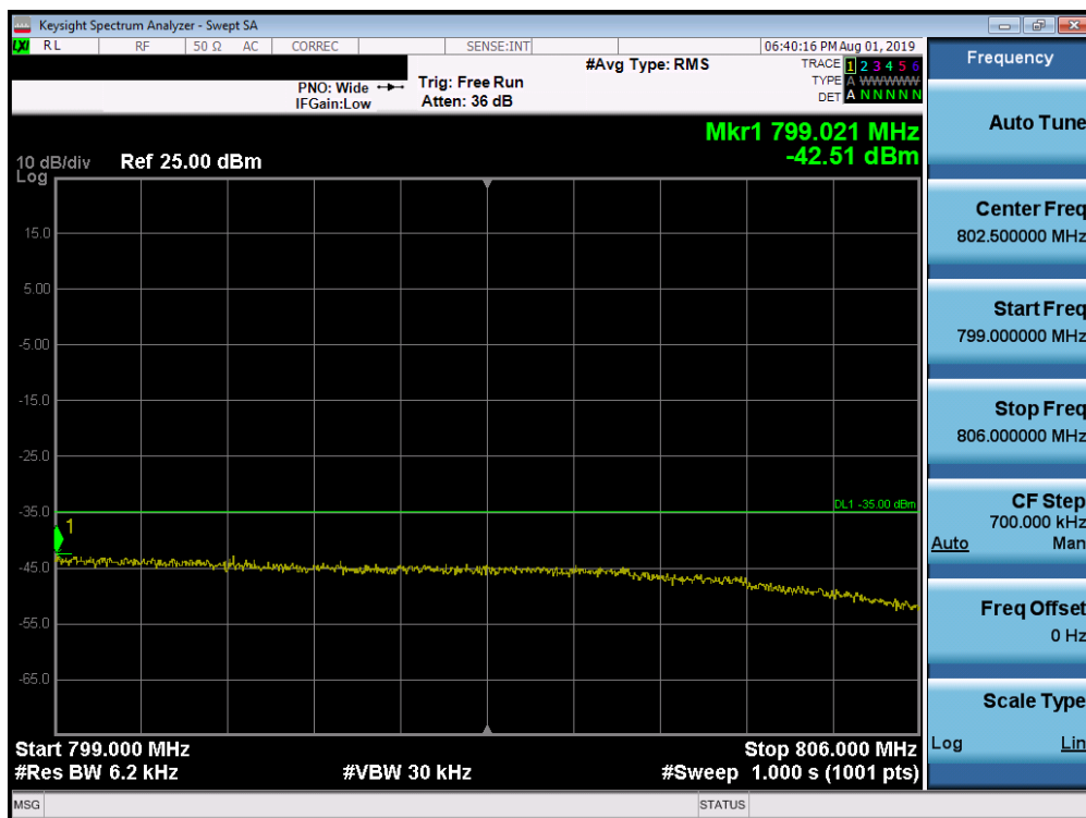
Plot 7-62. Upper Emission Mask Plot (LTE Band 14, 10MHz QPSK – RB Size 50)
