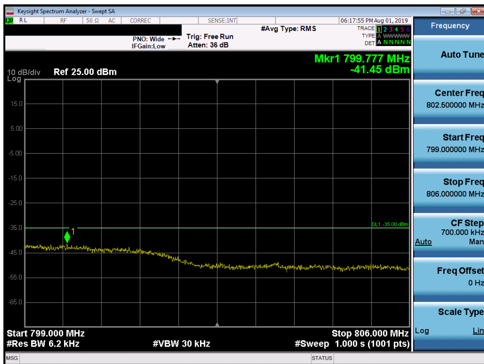
Plot 7-58. Upper Emission Mask Plot (LTE Band 14, 5MHz QPSK – RB Size 25)
