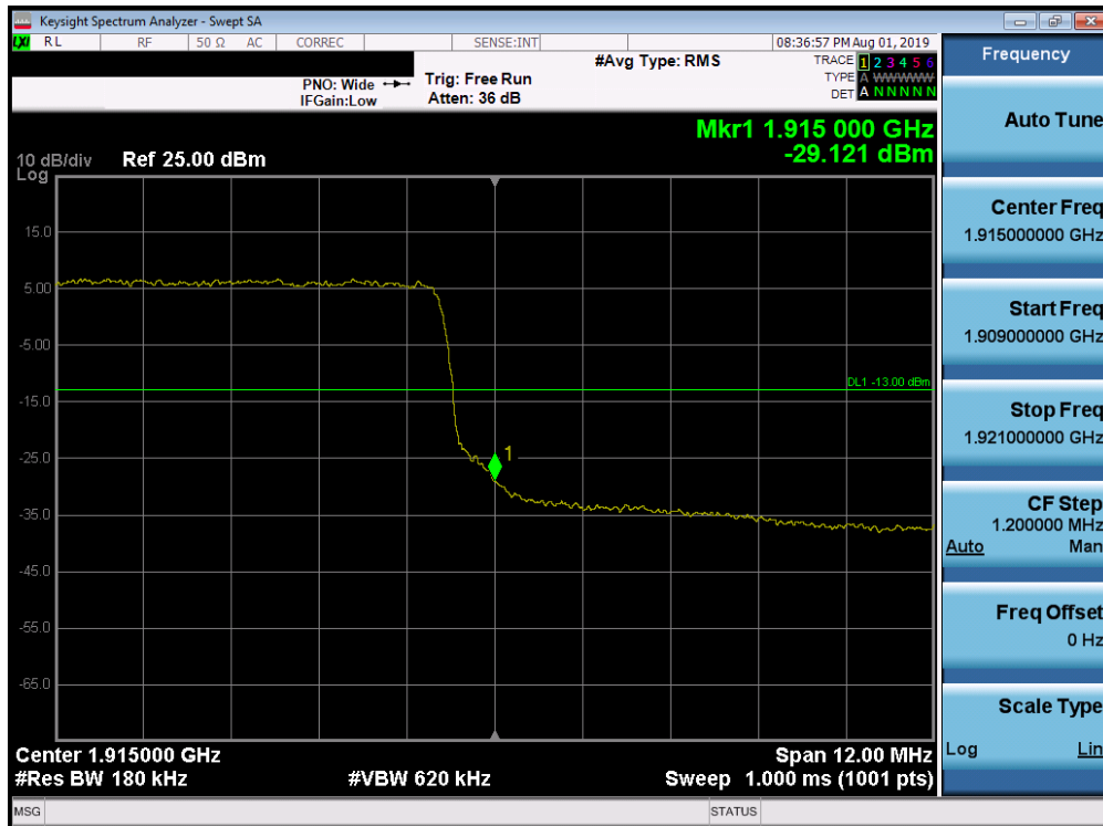
Plot 7-277. Upper Band Edge Plot (Band 25 - 15.0MHz QPSK - Full RB Configuration)
