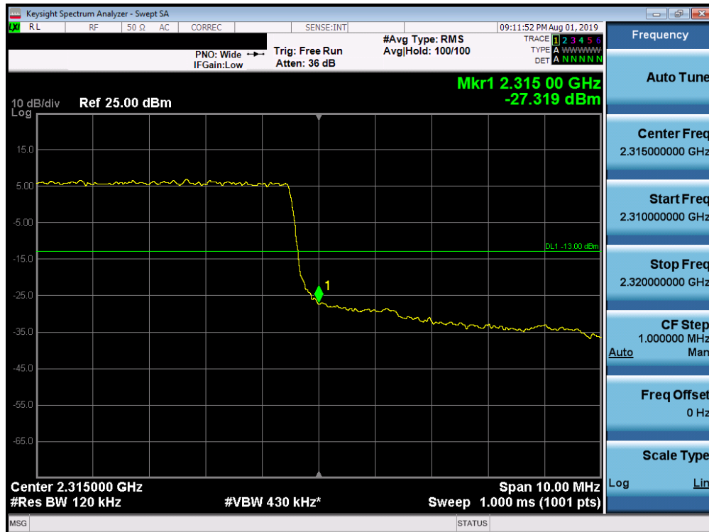
Plot 7-292. Upper Band Edge Plot (Band 30 - 10.0MHz QPSK - Full RB Configuration)
