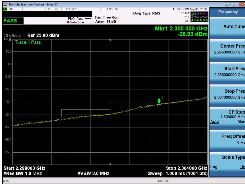
Plot 7-291. Lower Extended Band Edge Plot (Band 30 - 10.0MHz QPSK - Full RB Configuration)
