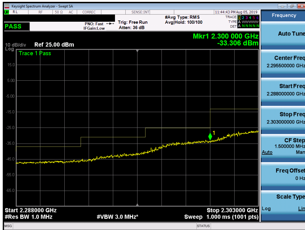
Plot 7-286. Lower Extended Band Edge Plot 2288-2303 MHz (Band 30 - 5.0MHz QPSK - Full RB Configuration)
