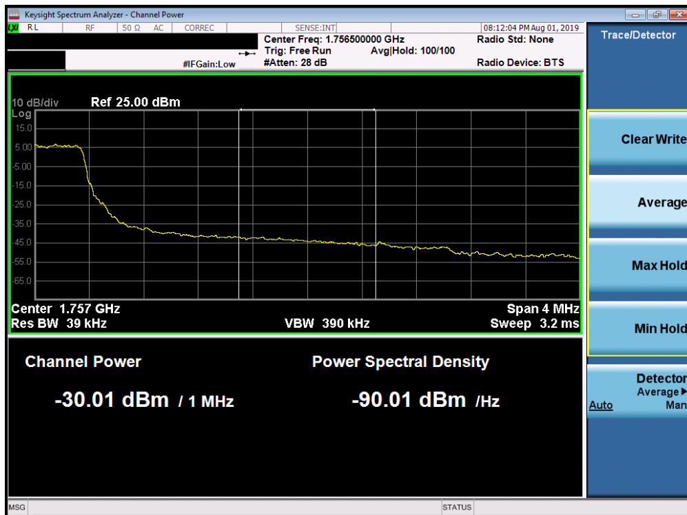
Plot 7-222. Upper Extended Band Edge Plot (Band 4 - 3.0MHz QPSK - Full RB Configuration)
