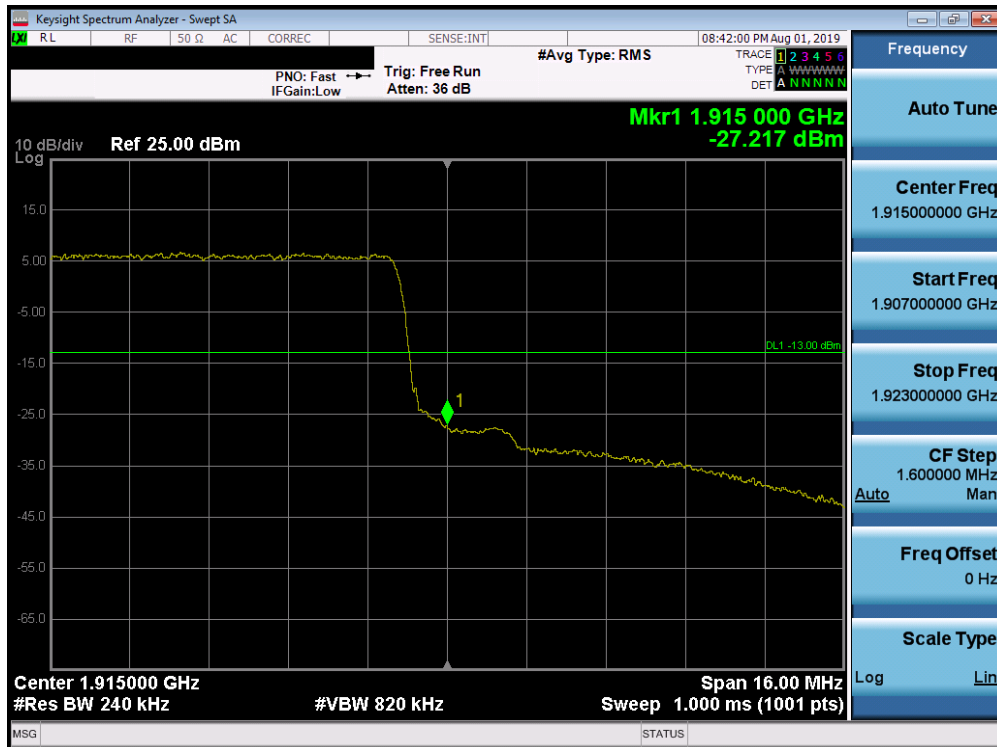
Plot 7-283. Upper Band Edge Plot (Band 25 - 20.0MHz QPSK - Full RB Configuration)
