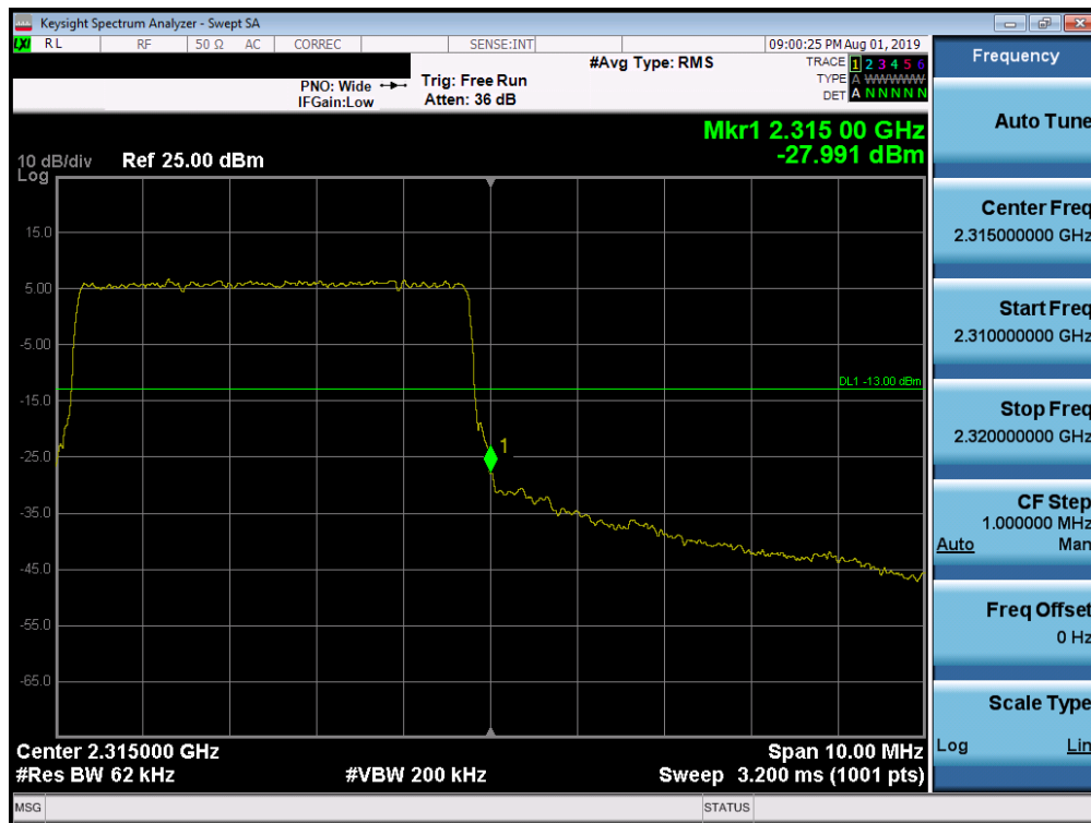
Plot 7-288. Upper Band Edge Plot (Band 30 - 5.0MHz QPSK - Full RB Configuration)
