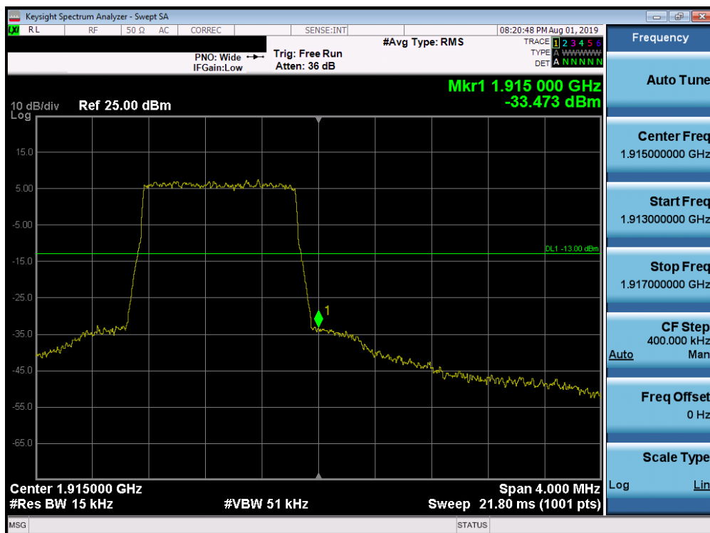
Plot 7-253. Upper Band Edge Plot (Band 25 - 1.4MHz QPSK - Full RB Configuration)
