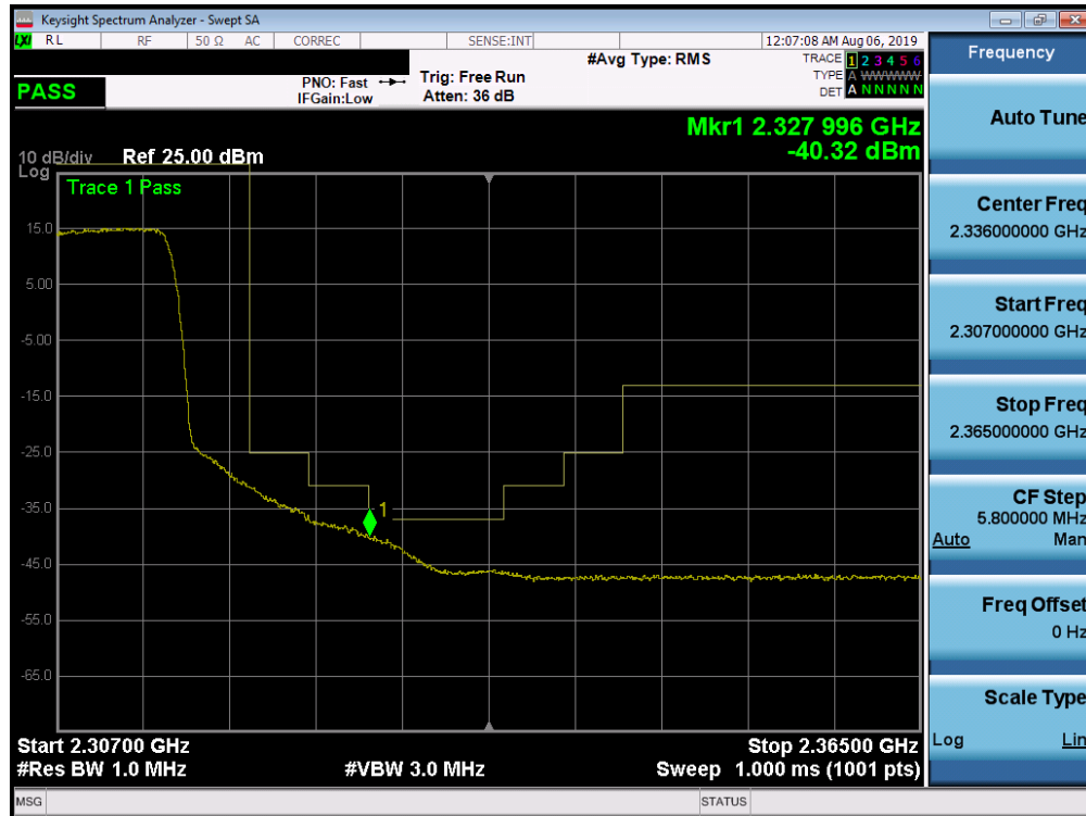
Plot 7-293. Upper Extended Band Edge Plot (Band 30 - 10.0MHz QPSK - Full RB Configuration)
