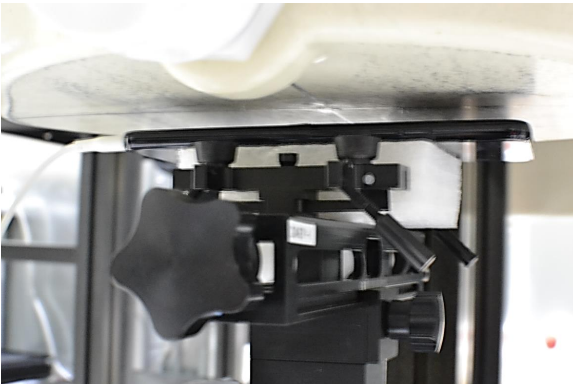
SAR Test Setup Photo 6: Back at 1.0 cm with Headphones
