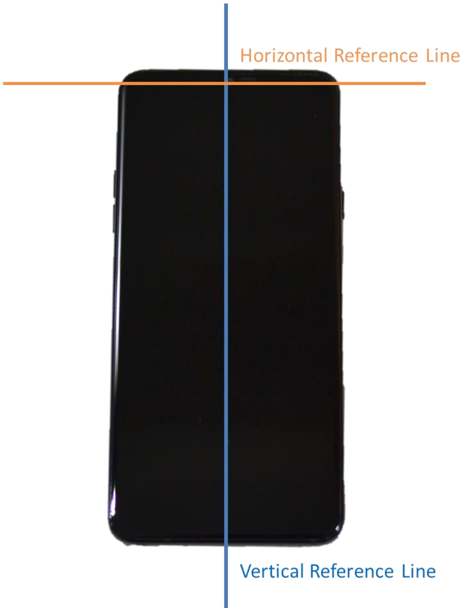
SAR Test Setup Photo 20: Vertical and Horizontal Reference Lines
