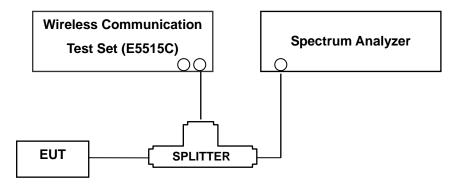
(Configuration of conducted Emission measurement)
