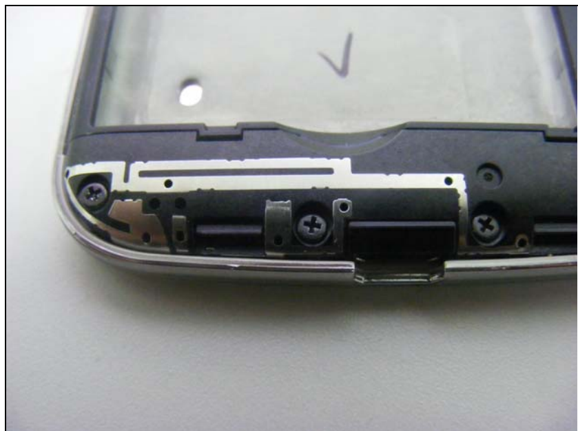
Top view of GSM&WCDMA Antenna
