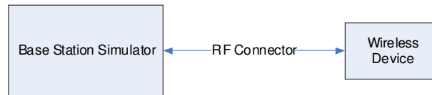
Figure 9-2 Power Measurement Setup
