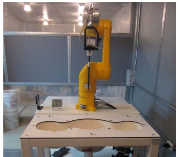
Figure 2.2 DASY5 Test System
