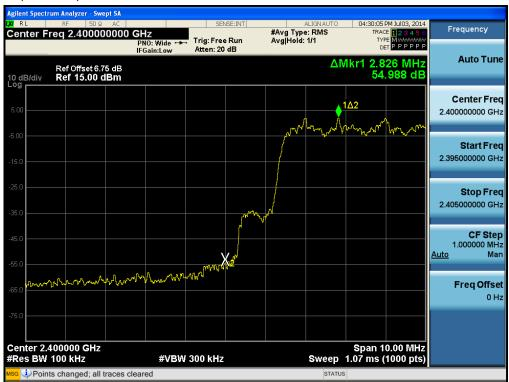
Test Plots with hopping (π/4DQPSK) Band Edges (High-CH)
