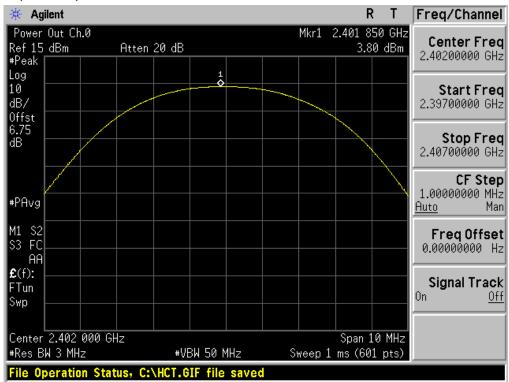
Test Plots (GFSK) Peak Power (Mid-CH)
