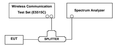
(Configuration of conducted Emission measurement)
