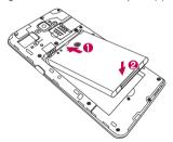
4 Align the battery cover over the battery compartment (1) and press it down until it clicks into place (2).
