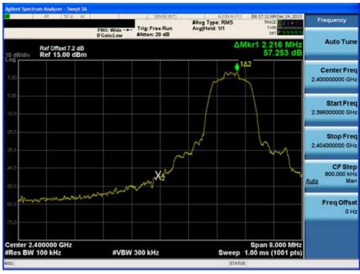
Test Plots without hopping ( $\pi$ /4DQPSK) Band Edges (High-CH)
