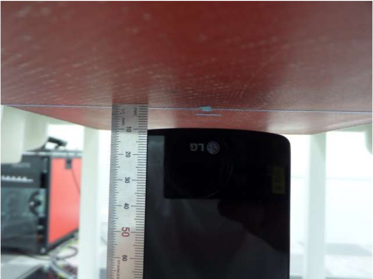
[Distance of 1.0 cm from the EUT]
