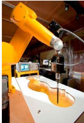
Figure 3-1 SAR Measurement System
