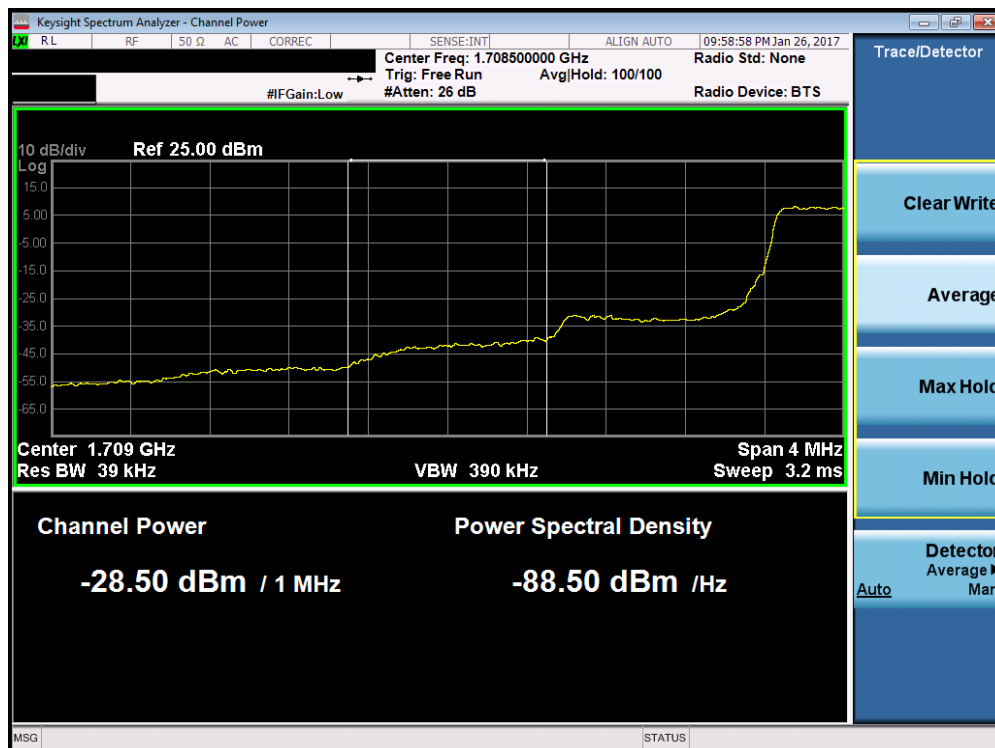
Plot 7-94. Lower Extended Band Edge Plot (Band 4 – 1.4MHz QPSK – RB Size 6)
