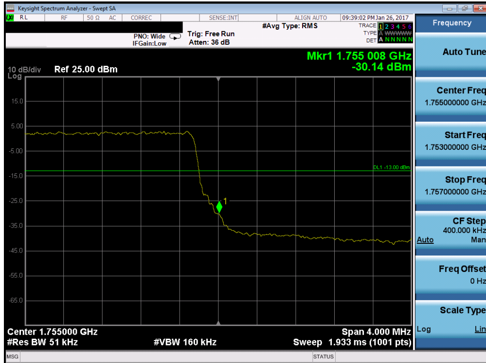
Plot 7-103. Upper Band Edge Plot (Band 4 – 5.0MHz QPSK – RB Size 25)
