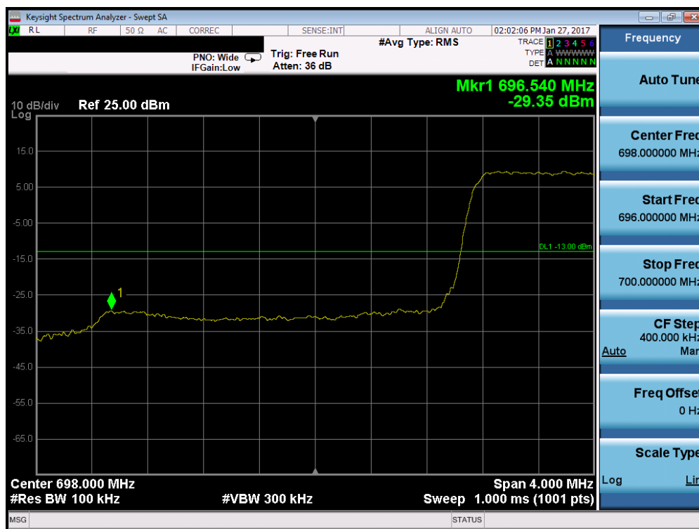
Plot 7-79. Lower Band Edge Plot (Band 12 – 3.0MHz QPSK – RB Size 15)
