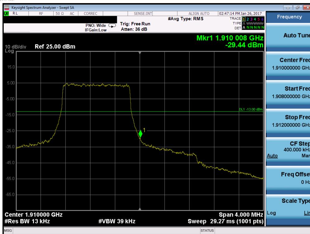
Plot 7-119. Upper Band Edge Plot (Band 2 – 1.4MHz QPSK – RB Size 6)
