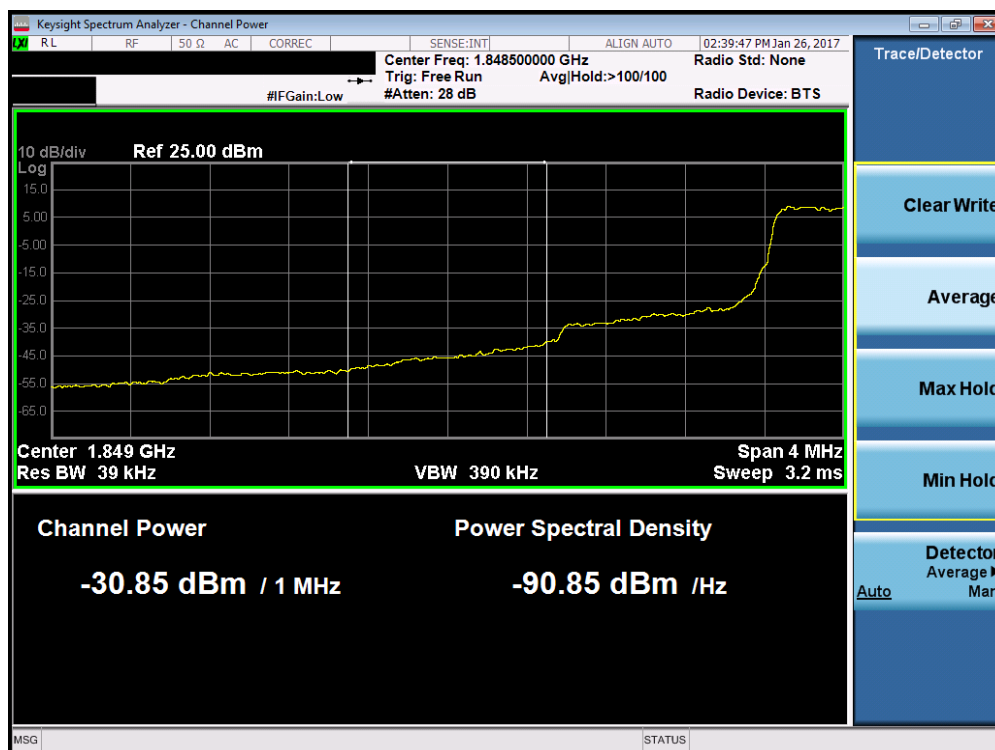
Plot 7-118. Lower Extended Band Edge Plot (Band 2 – 1.4MHz QPSK – RB Size 6)
