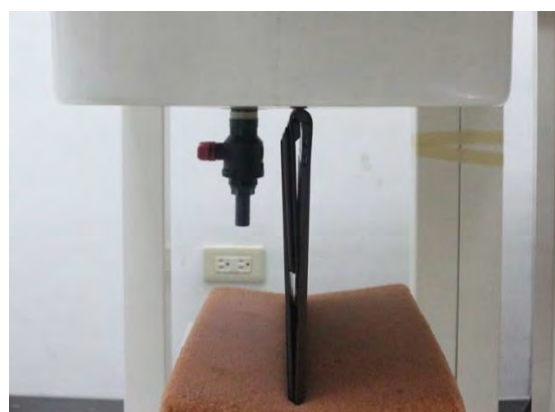
Fig.4 EUT Top side to flat phantom
