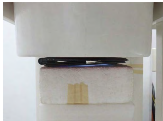
Fig.3 EUT Back side to flat phantom
