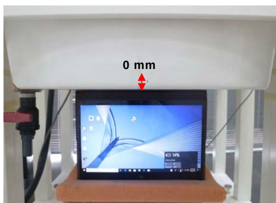
Fig.4 EUT Top side to flat phantom
