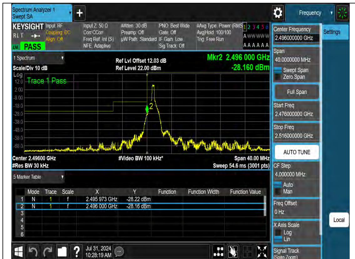
N41-20M-Bandedge-H-DFT-s-OFDM-Pi2 BPSK-Outer Full
