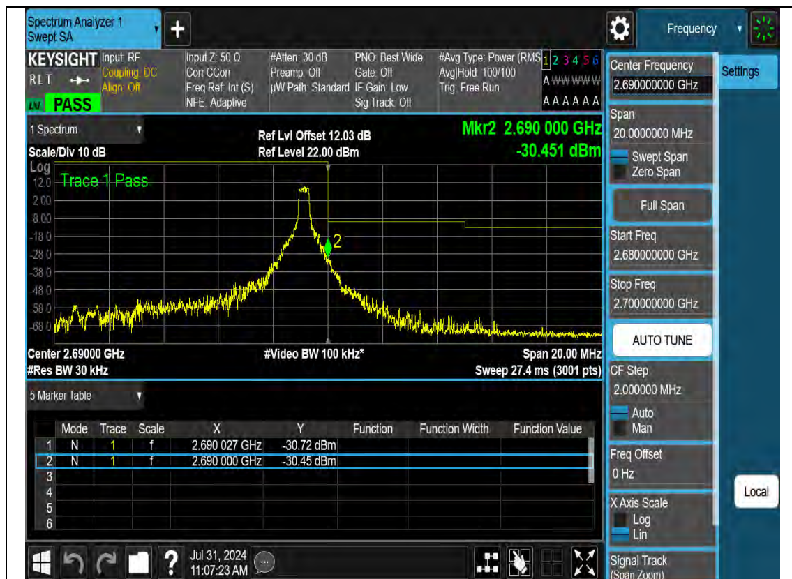
N41-15M-Bandedge-L-DFT-s-OFDM-Pi2 BPSK-Outer Full
