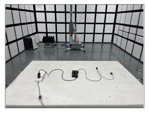
Radiated emission test: Frequency Range< Above 1GHz >
